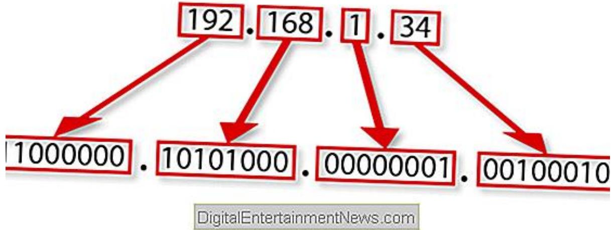
Slika 14.Prikaz IP adresiranja, Izvor: <https://hr.digitalentertainmentnews.com/how-do-ip-addresses-work-983840> (17.01.2022.)
